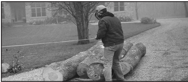
Fig. 23—Attaching choker or winch strap
