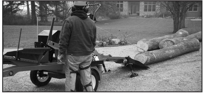
Fig. 24—Winching First Log
