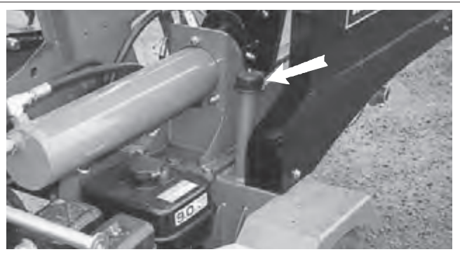
Fig. 47 HYDRAULIC OIL LEVEL (Typical)
