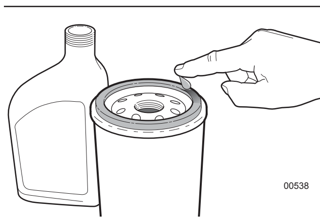
Figure 60 —Apply a light coat of hydraulic fluid to the filter seal
