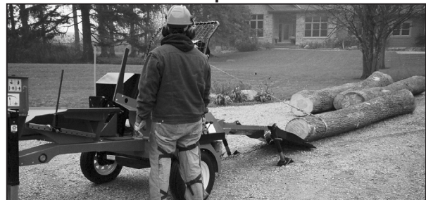
Winching First Log
