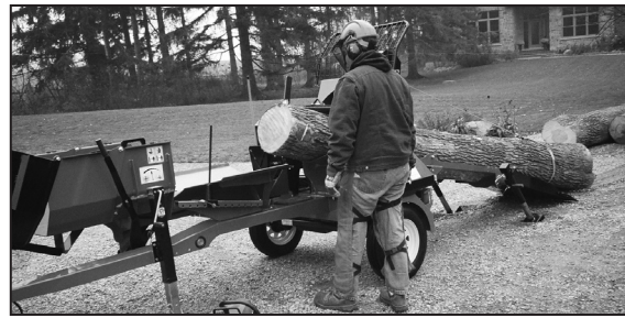
Winching to Cutting Guide
