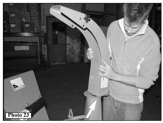
20. Install second half of Spacer Rings. Slide the lower portion Ring beneath the slotted lip of the Upper Rotor Housing while at the same time aligning the holes of the upper Ring with the holes in the Discharge Chute. *Photo 24*
