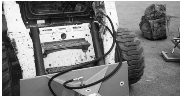
Safely route hoses
