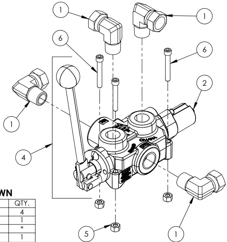
**VALVE AND FITTINGS PARTS BREAKDOWN**
