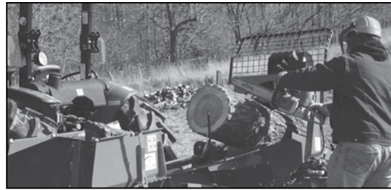
Winching to Cutting Guide
