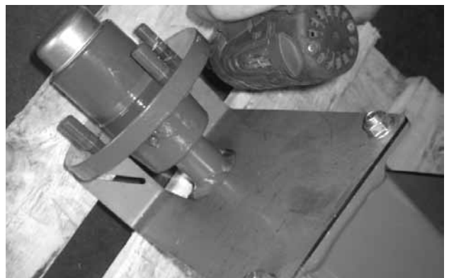
Remove Fasteners from Axle Shipping Brackets
