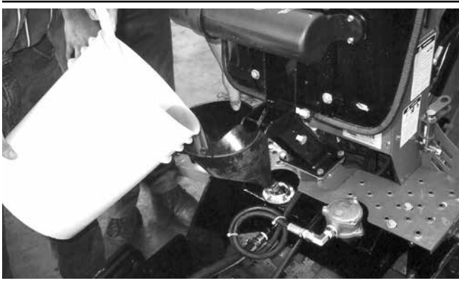
Fig. 8 – Fill Reservoir with Oil
