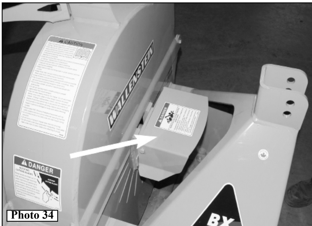
27. Locate PTO Guard and swivel up. Photo 34
